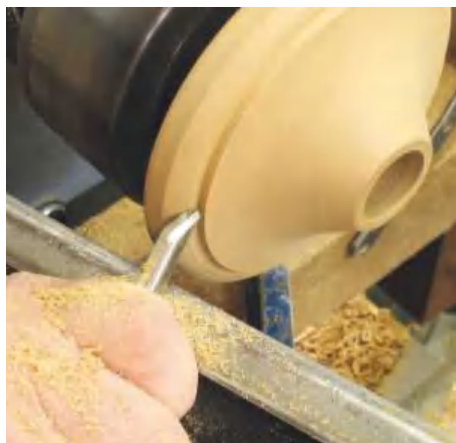
▲ Pic.14 Rounding over the bottom section of the base will be aesthetically pleasing. The grain of the timber is going in a different direction than spindle work so the tool works up the bead rather than down; this will give you a superior finish
